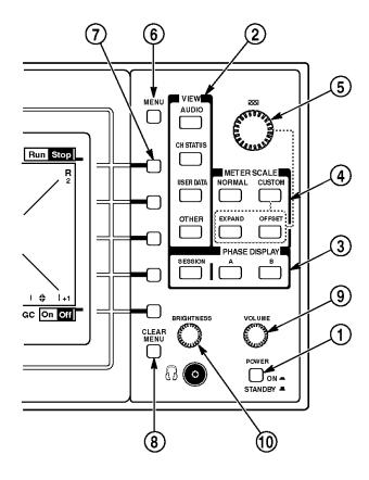
Figure 14: 764 front-panel controls
